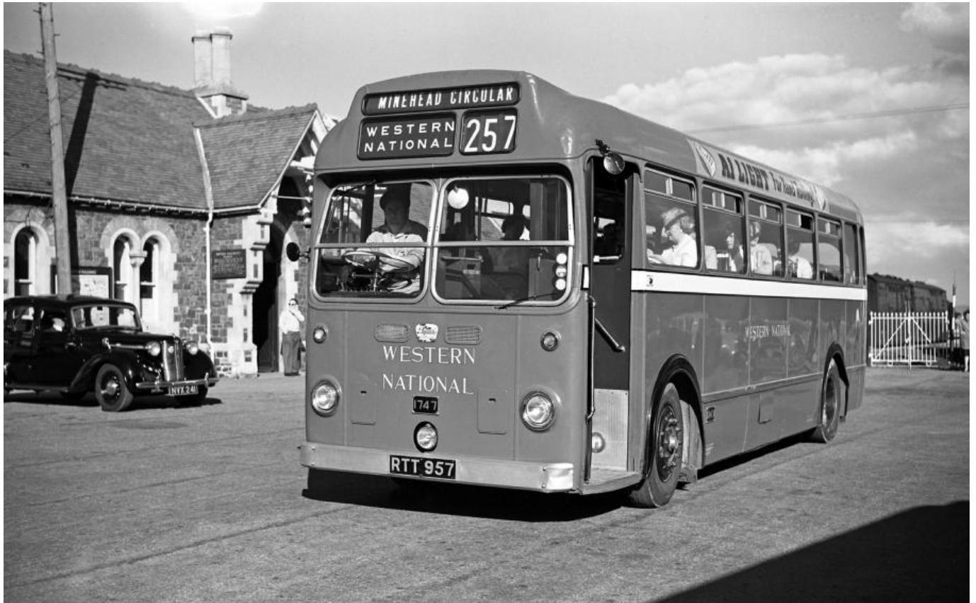
Western National 1747 (RTT 957), a 1955 Bristol LS5G with 45-seat Eastern Coach Works body, operating a Minehead town service. A white steering wheel reminds the driver that this vehicle is 8 ft wide. The chipped Bristol/ECW badge and dented bumper suggest this otherwise immaculate bus is not new. The Austin 10 car has a 1949 Essex registration. Minehead railway station closed in 1971 and the West Somerset Railway reopened it in 1976. Photographer Roy Marshall, copyright The Bus Archive, ref. RM02/14748.
